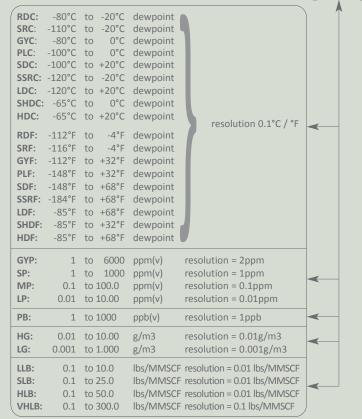
NOTE: ppm, ppb, g/m3 & lbs/MMSCF ranges are stated at atmospheric pressure. Model AMT Transmitter can be configured to provide corresponding ranges for operation at other constant pressure. This must be stated at time of order.
